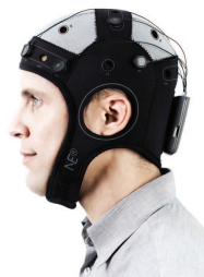
High resolution tCS with simultaneous EEG monitoring (available from StarLabs)
